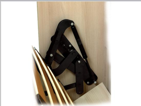
Special design of gas strut hinge with gas strut being in a safe position while the cabinet is open (bed position). Gas strut hinge can be tightly fixed to the cabinet panels while only using wood screws.
